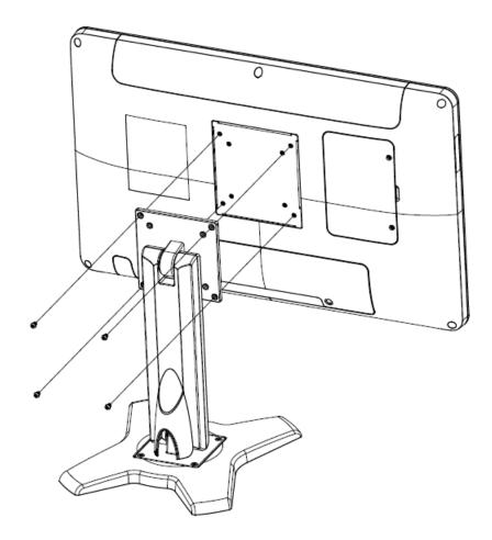
**Step1.** Position VESA Mount on both sides, matching the holes on the system. **Step2.** Insert and fasten 4 screws on each side of the monitor to secure Mounting brackets.
