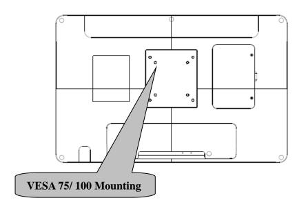
Suggested Screw type for mounting **Note:** 4 pieces of M4 x 6mm screws (P/N: E1933050611R)
